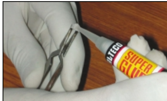
Fig. 4 Cyanoacrylate glue applied to non-adhesive side of tape.
